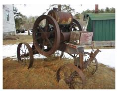
The engine came from a farm near Alpha, WI. This picture shows one of the unique features of the engine. The cart is actually the frame of the engine.
