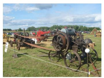
The Lightning Balanced engine now runs very well and belt powers it's companion restored Kansas City Hay press to bale straw.
