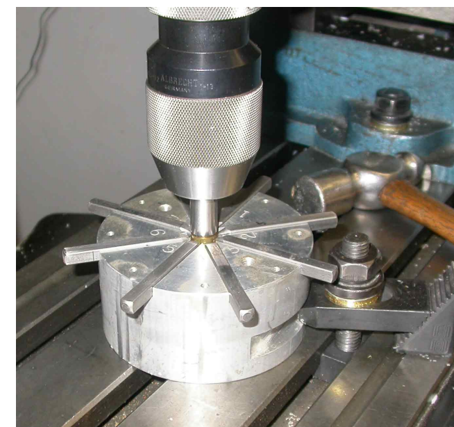
Fixture for Stamping Numbers on Needle Head Needle Head in the middle held down by steel pin in Chuck, just give each stamp a hit and all done.
