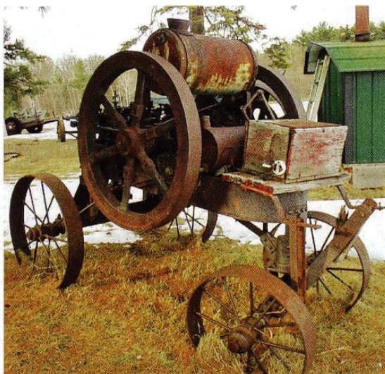
The 10 hp Kansas City Hay Press Lightning Balanced Engine as it looked when Marvin Hedberg acquired it.
