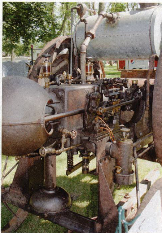
A close-up of the real Lightning (right). Notice the valves under the cylinder. Serial number 9 on the replica build plate honors Marvin's friend Morris Blomgren (below).
